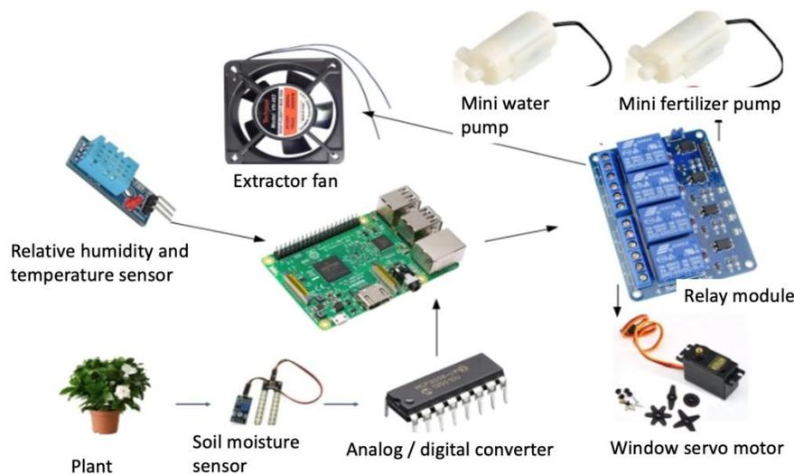
Figure 2. Sensor and actuator connection diagram.
